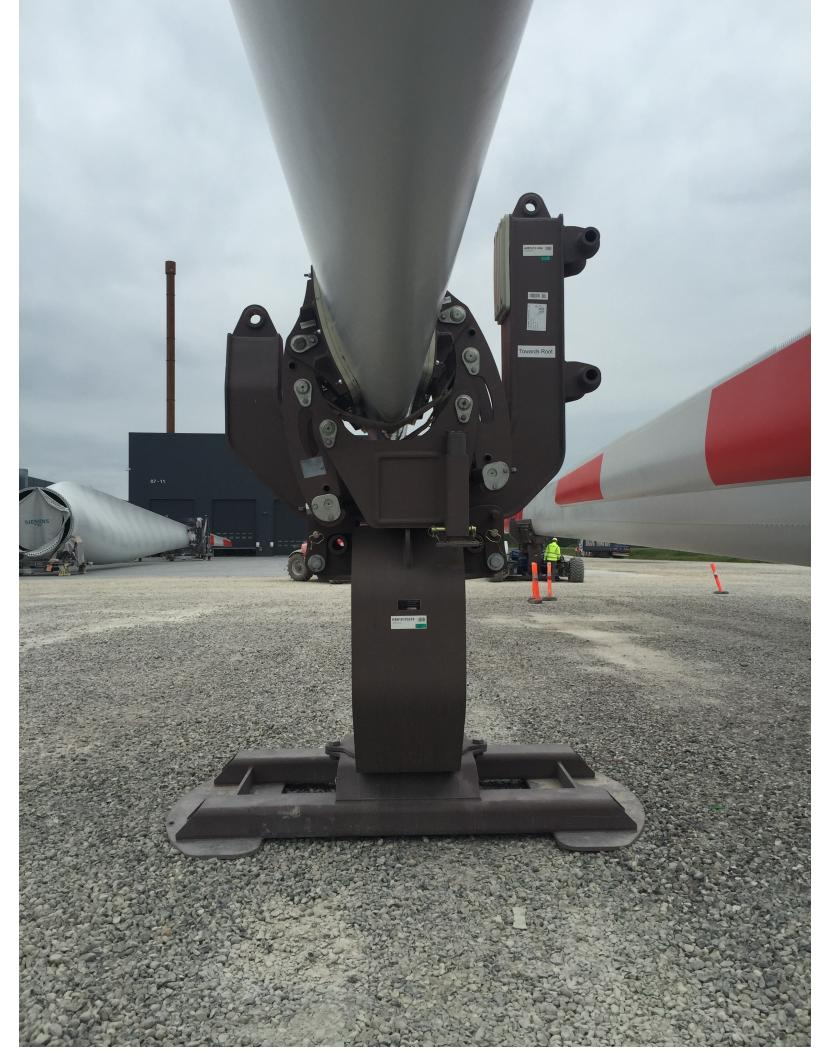
PRE-FABRICATED STEELWORK STRUCTURES AT ROOT & TIP END INCORPORATING THE STANDARD FIXINGS USED BY SIEMENS.
