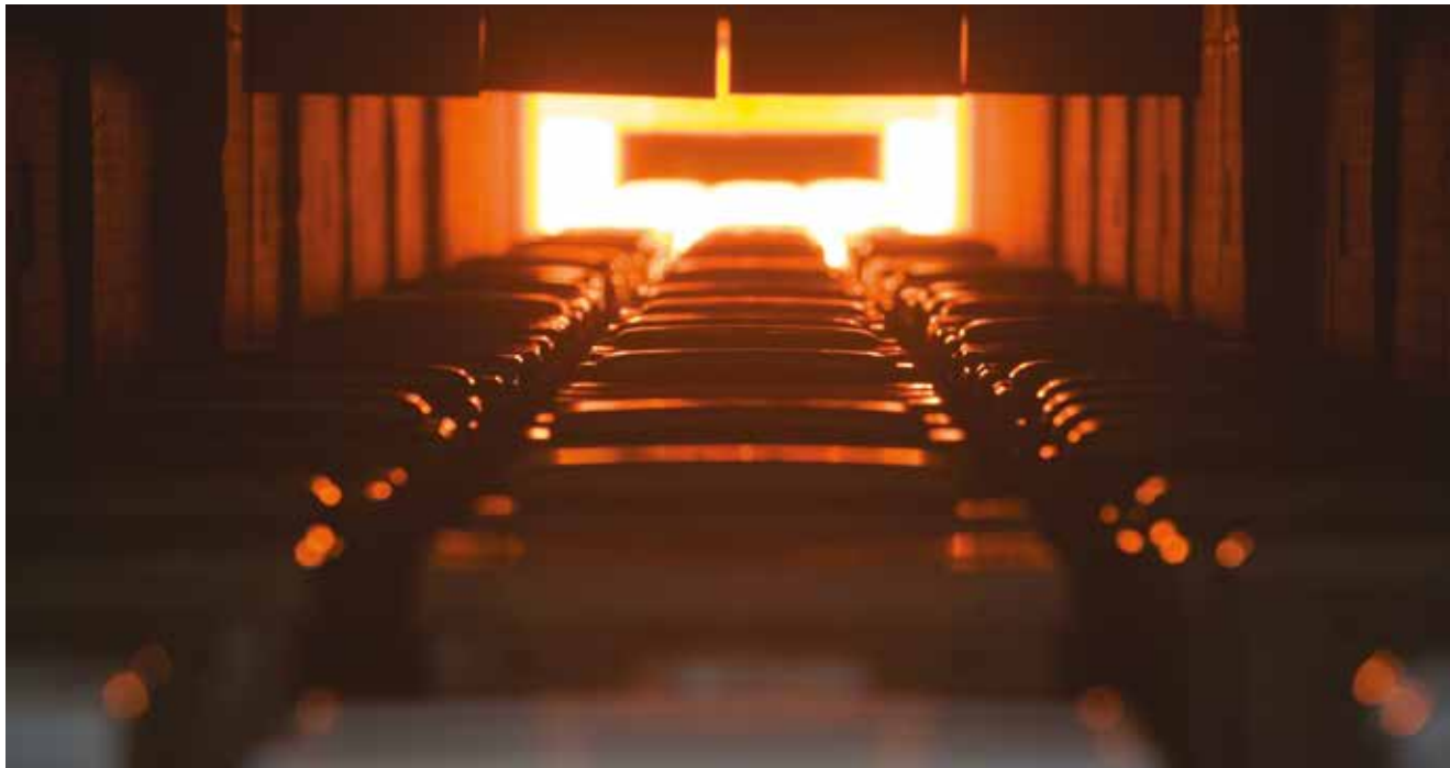
Ceramic ware being fired in one of the long tunnel kilns at the Armitage factory
