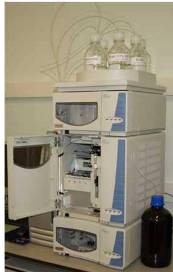
Figure 14.30 - an HPLC system
