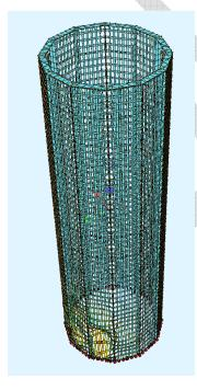
The fist buckling factor is 4.28, corresponding to an instabilization of a bottom perforated steel cassette in correspondence of the leeward side, where the largest compression stresses are located.
