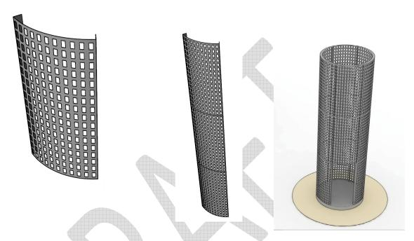
Three steel cassettes, put on top of each other and connected with flat plates, form a full height element.
