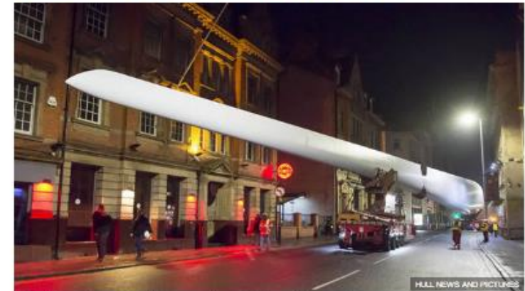
Traffic lights and lampposts had to be removed so the turbine could be moved
