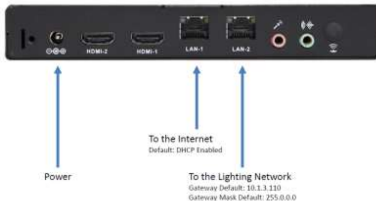
Figure 7: ActiveSite Gateway connection to the Internet and to the lighting network.
