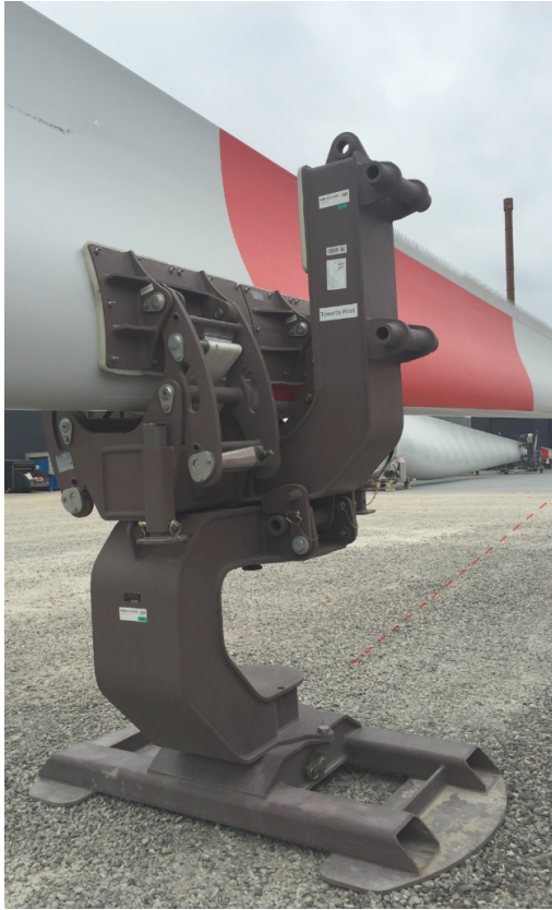
Siemens clamp used to hold blade in position:
