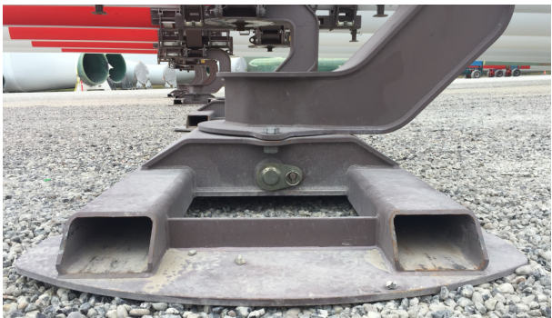
Existing connection detailed copied to connect clamp to tripod:
