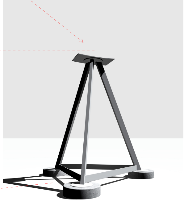
Steel tripod structure: - support off spreader structure. - clamp used to hold blade.
