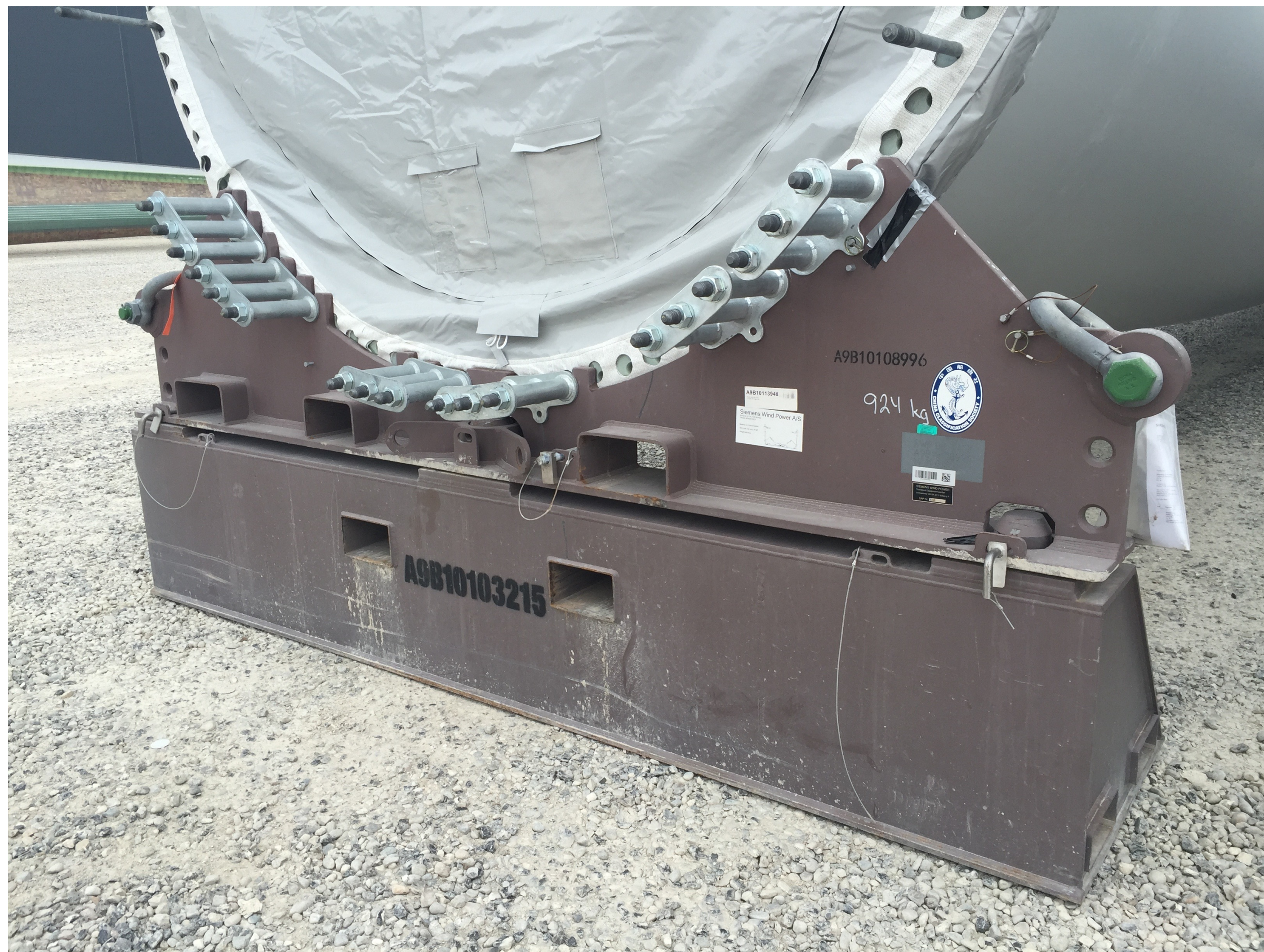
PRE-FABRICATED STEELWORK STRUCTURES AT ROOT & TIP END INCORPORATING THE STANDARD FIXINGS USED BY SIEMENS.
